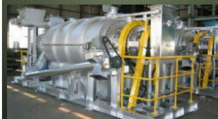
K2 CARBONIZATION PLANT 20 TONS PER 8-HOUR SHIFT BASED ON DRY WEIGHT BIOMASS
